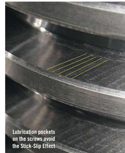
types with defined loads. Therefore it is crucial for us that the performance of our lifting jacks is not compromised by lubrication problems when we reach the maximum contact pressure per unit area” says Clinton Capelli, Engineer at Vector Lifting which supplied one of the largest lifting jack installations
